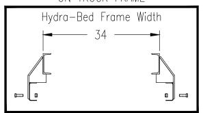
Bolt 2 1/2x2 1/2x54" tube to factory frame risers. Center Hydra-Bed 10" from each end of tube. Weld Hydra-Bed frame to tube risers. Hydra-Bed frame will be resting on tube and between risers.
